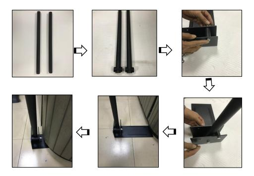
Step 2: Insert the upper&lower support arm into the center couple piece. Then slide it into the support arm which already connected with mounting bracket. Then press the decorative Small Black Dome Caps over the heads of all the exposed screws. Note: the 3pcs center couples are used singly or in combination to small spas and big spas(Spas' size from 1.5 m to 2.5 m).
