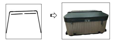
Step 3: Lay the Cover Lift on the spa cover. using the Self Tapping Screws to fasten the Support Arms and Coupler Pieces together. Slide the folded cover into support arms, Finally push the cover down and the cover storing neatly out of the way.
